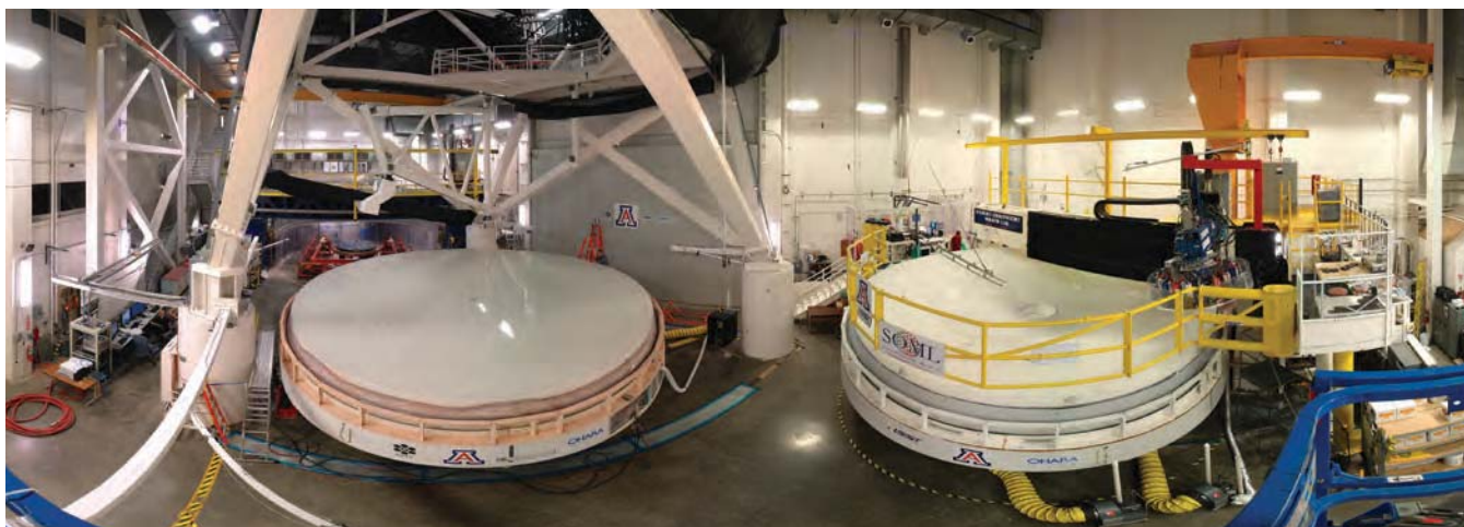
Steward Observatory Mirror Lab. Two 8.4-meter mirror castings appear side by side in this wide angle panorama view inside the Lab's mirror polishing area. On the left undergoing optical testing is the first mirror blank (of eight planned) cast for the Giant Magellan Telescope Observatory (GMTO). On the right is the mirror casting for the Large Synoptic Survey Telescope (LSST), undergoing polishing of its dual curvature upper surface.
