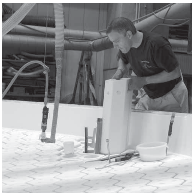
RESEARCH: Randy Lutz, Manager of the Steward Observatory Mirror Lab Casting group, installing the last of the 1020 individual hexagonal columns for the 6.5 meter diameter mirror casting mold. The finished mirror will be installed in a new telescope to be built at San Pedro Mártir, Baja California, Mexico. Courtesy of Ray Bertram, Steward Observatory
