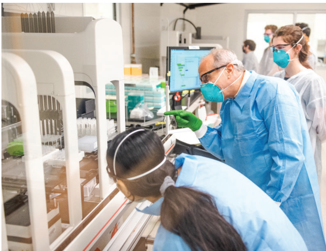
High-throughput automated liquid handler currently used for the COVID-19 testing at the ASU Biodesign Clinical Testing Laboratory.
